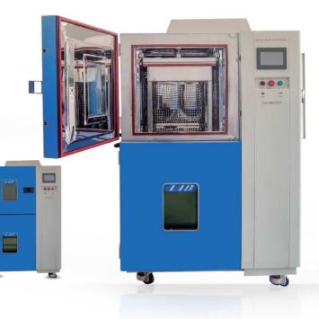
LIB 3TS series thermal shock test chamber is just one chamber for test room. It circulates cold and hot air through the pneumatic damper on the left and right sides. This design makes external size smaller, and the 3TS series thermal shock chambers can be pre-heated and precooled to achieve faster temperature change.
